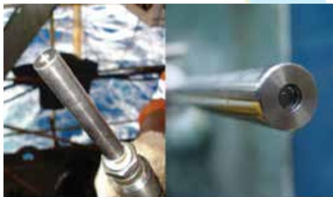
**FRONT SURFACE UV FLUORESCENCE PROBE**
