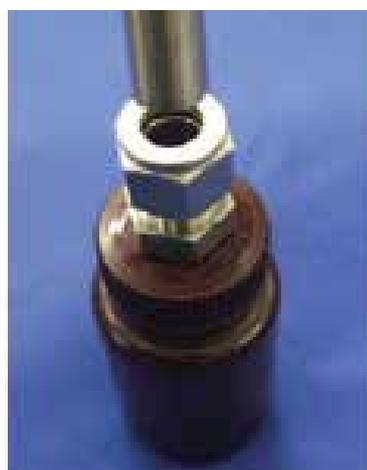
Prepare the zero or span solution, pour into the calibration bottle, insert the probe and calibrate the unit.
