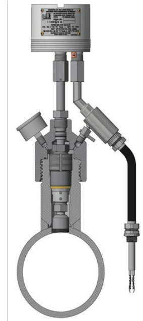
Microcor Transmitter on an Access Fitting
