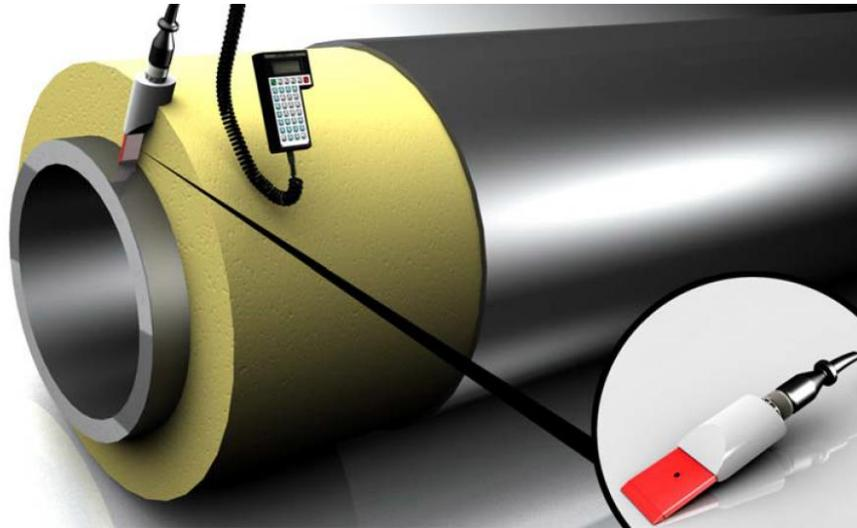
Figure 8. Example of Corrosometer probes inserted in the insulation with the handheld to measure the corrosion rate
