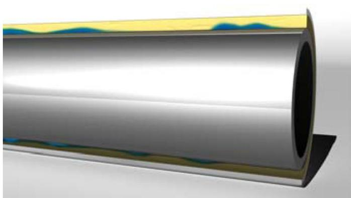
Figure 2. Moisture trapped in the insulation can create a corrosion cell on the pipe surface
