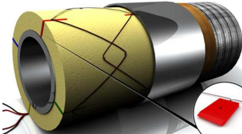
Figure 6. Example of probes inserted at 4 clock positions around pipe
