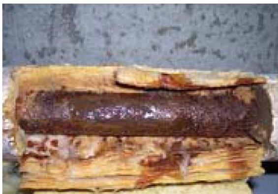
Figure 1. Severe outer pipe wall corrosion due to CUI
